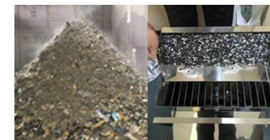
Research on optimization of ASR recovered resin recycling process. Left photo is ASR and right photo is resin recovered from ASR.
